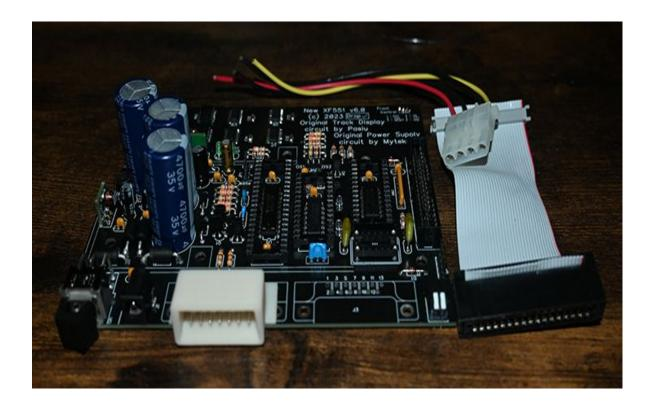
If you use a sonic cleaner make sure you give it plenty of time to dry out all the nooks and crannies. You should be finally ready to install the chips and OSC. This board does not need the heat sink that was in the original Atari XF551, I would store it just in case, or use it for an ornament.
