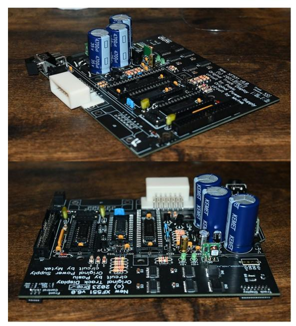
Note that the 5V regulator assembly is soldered like a 7805 with the parts facing the big caps. The 12V regulator assembly faces away from the big caps.
